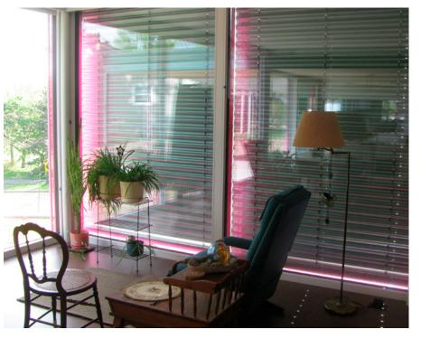
**Right, clockwise from top left:** The bird-friendly glass used for large windows has an imprinted web-like pattern of ultraviolet pigment. Birds see it easily, but to humans it's visible only at a limited reflection angle from outside the window; A close up of the web pattern; Adjustable blinds outside east, south, and west windows block heat on summer days. Slats can be adjusted to allow views while screening unwanted heat.
